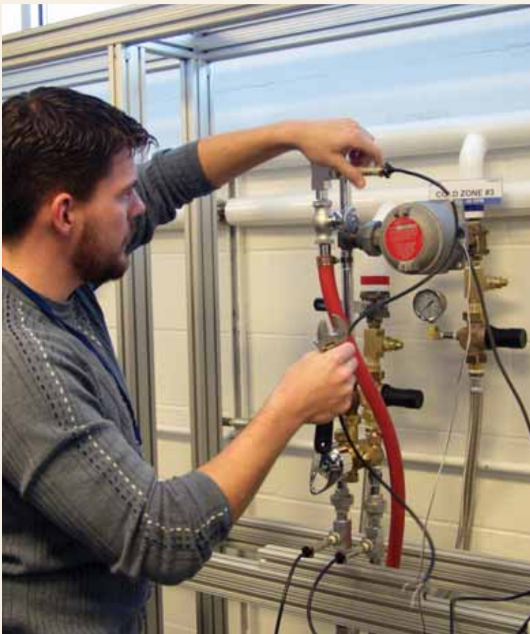
Chicago Faucet Engineer Ryan Schlangen attaches a pressure transducer to a shower valve in order to monitor results using their data acquisition system.
