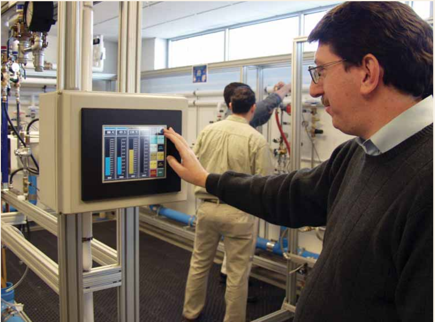
Chicago Faucet's Product Compliance and Testing Coordinator Larry Himmelblau demonstrates the test lab's touch screen controller that allows engineers to vary pressures to a particular zone, trend a particular period of time, monitor pressures and flows, clear and monitor alarms and see the entire system status with a touch of a button.
