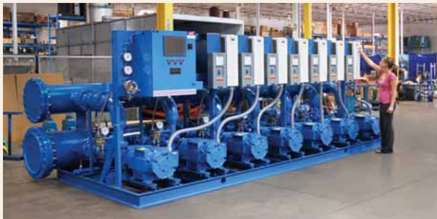
Inside Sales Engineer Emilee Jones performs some final checks before one of the largest booster systems ever manufactured by Metropolitan ships to Chicago's McCormick Center to serve the west end expansion currently taking place there. The system utilizes seven 50-HP end suction pumps capable of pumping 4200 gallons per minute at 243' total dynamic head.
