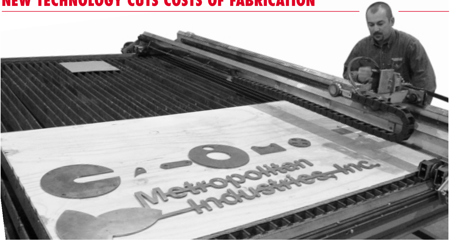
Bob Svoboda demonstrates the capabilities of the new plasma cutter as he displays Metropolitan's logo cut from a sheet of steel. Using CAD\CAM computer software, the plasma cutter will cut according to exact specifications in a drawing.
