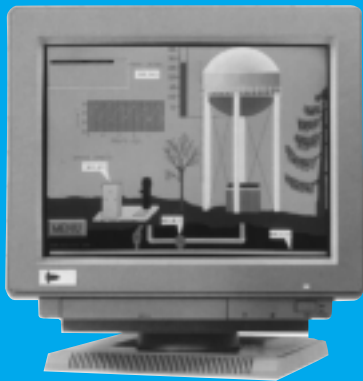
Monitor pump reservoirs, valve vaults, overhead tanks, sewage lift stations, etc., all from a remote location.
