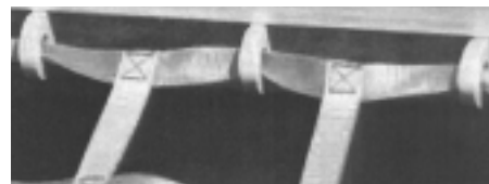
Track system allows nets to slide to the side without disassembly.
